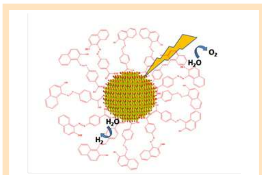
Figure 2: Water is split to release hydrogen and oxygen in the presence of the composition exposed to solar light.
