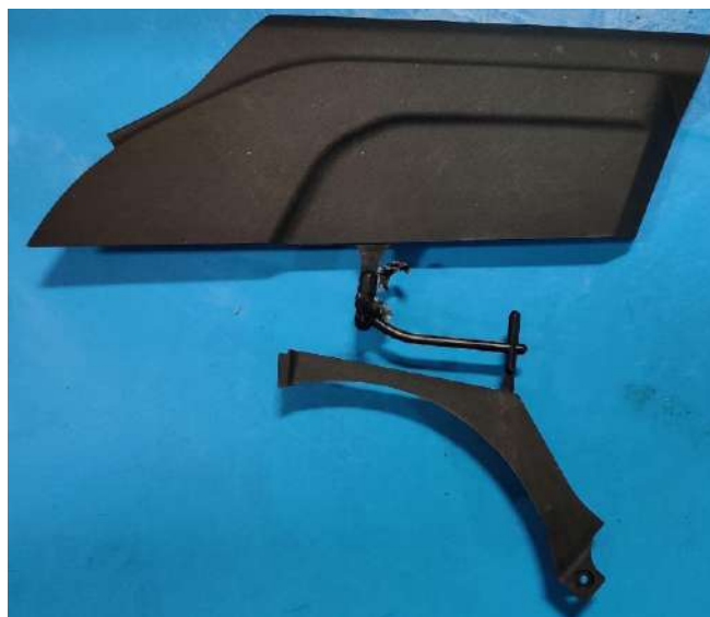
Figure 2: Long glass fiber thermoplastic composite molded structural automotive part made from decontaminated recycled PPE material
