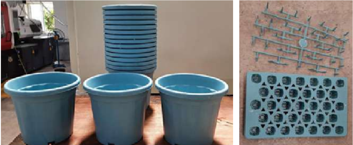
Figure 1: Garden pots & plant grower trays made from decontaminated recycled PPE material
